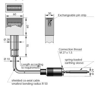
Particular characteristics TR 15/TR 25 The charging generators Tristat TR 15 / TR 25 suply an adjustable high-voltage of approx. 22 kV<sub>DC</sub>. The units are available in either positive or negative polarity. In case of the TR 25, the voltage set is displayed on the integrated measuring instrument. The high-voltage can be steplessly adjusted on a potentiometer. The Tristat TR 15 / TR 25 charging generators can be pulsed using an external control.
