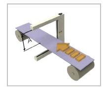
Distance B to an earthed machine part must be greater than the distance A.
