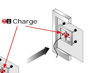
Typical applications for In Mould Labelling primarily exist in injection moulding, e.g. in food packaging (for the application of product labels) or in plastic containers of all types. During fixation of the label in the injection mould, the dielectric properties of the plastic are exploited in order to apply a defined charge to the label. This charge will allow it to be fixed in the grounded injection mould.
