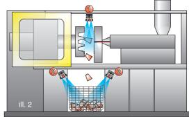
Below the mould, above the edge of the collecting container, blowing from one or two sides
