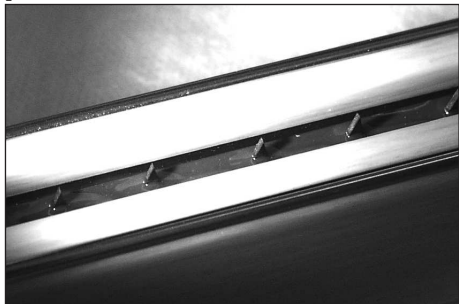
Ionizing pins made of silicon
