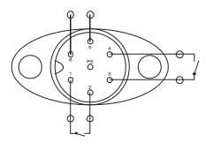
Contact load max. 24 VAC / 35 VDC, max. 50 mA
